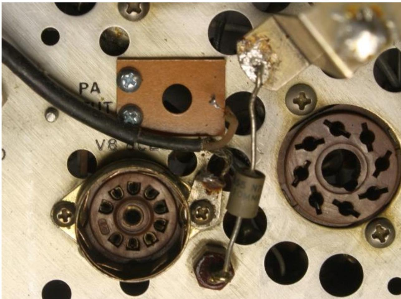
(15) Try if you can easily bend the center conductor of the small coax cable to a place right between the two new screws. If you can, then go to (17).
