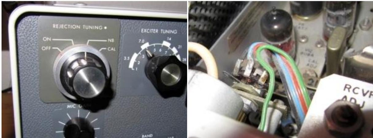
Here you can see the concentric former rejection tuning and power switch, and the RIT potentiometer mounted on the bracket that formerly held the variable capacitor.
