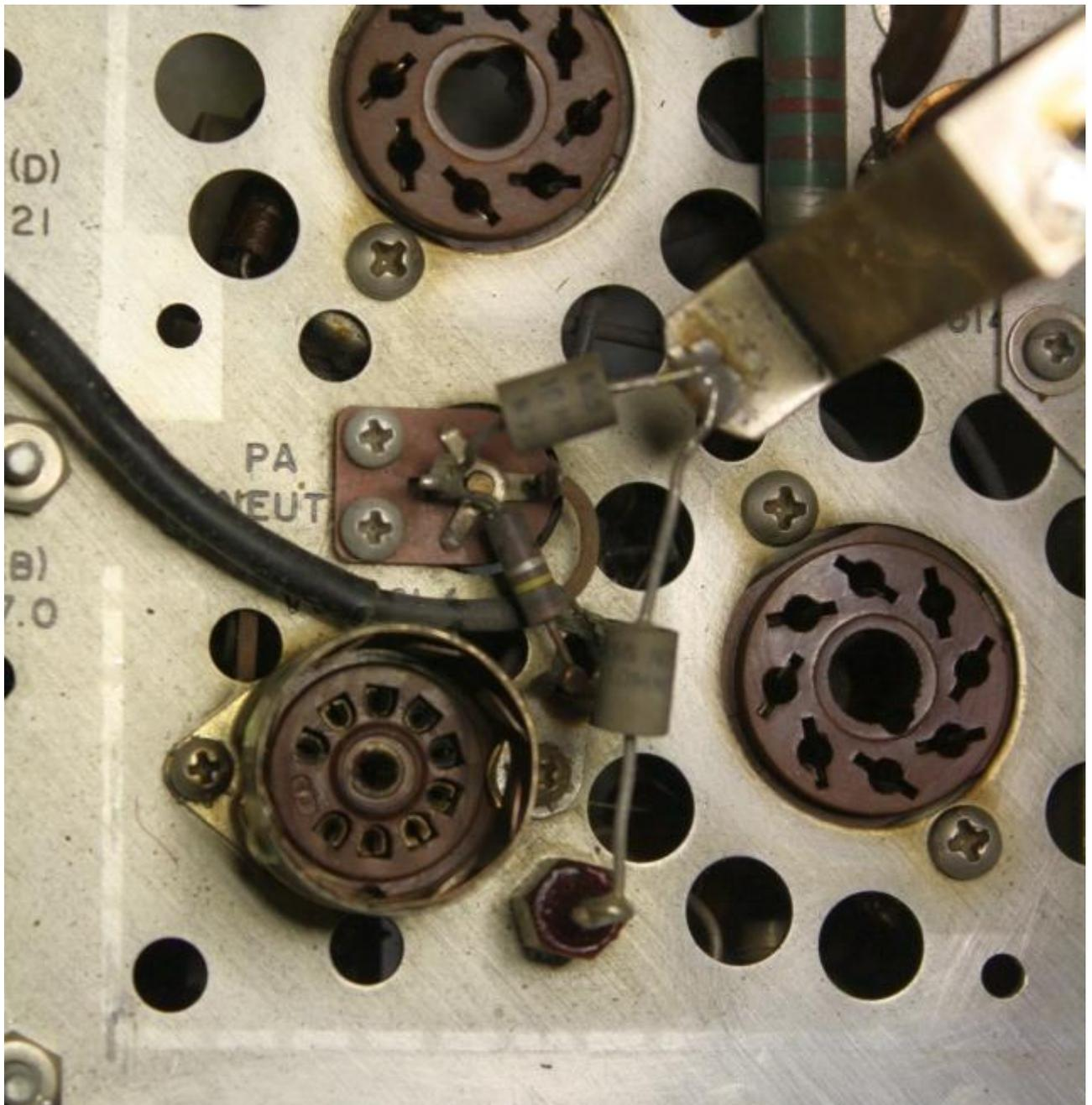
(12) Unsolder the inner conductor of the small piece of coax cable, the 100K resistor R127, and the 10 pF capacitor C183 from the small neutralizing capacitor C148. Then remove the two screws and capacitor C184. Now it should look like this:
